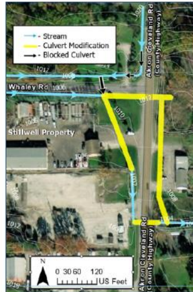
Akron Cleveland Rd Drainage
