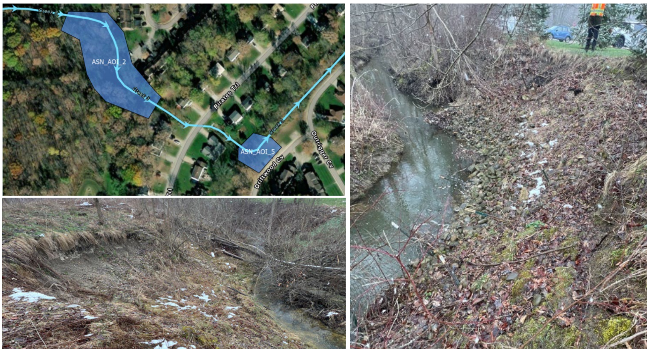
Right: Looking downstream - right bank erosion at ASN_AOI_5.
