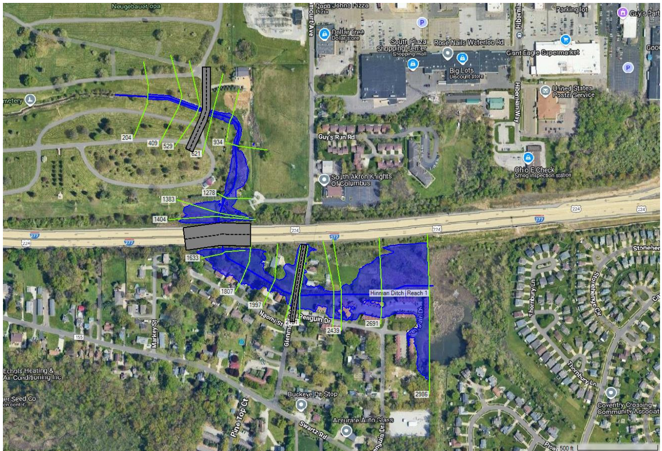
Figure 3 Existing Conditions 100-Year Water Surface - HEC-RAS Model
