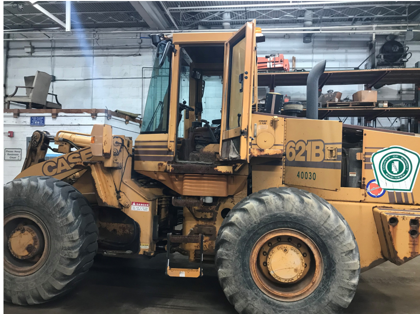
Loader 40030 sitting in the weld bay with no engine and rust visably showing on its body.
