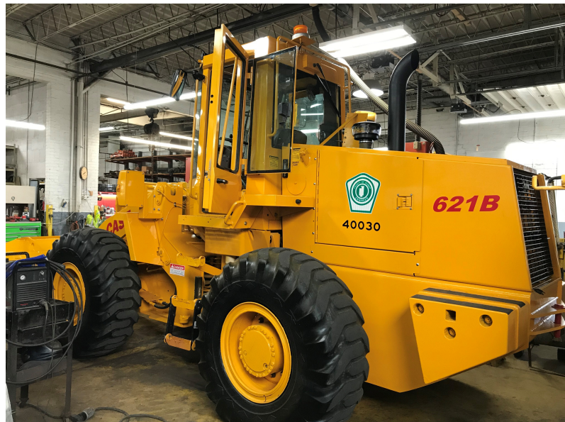
40030's bodywork completed and engine reinstalled.
