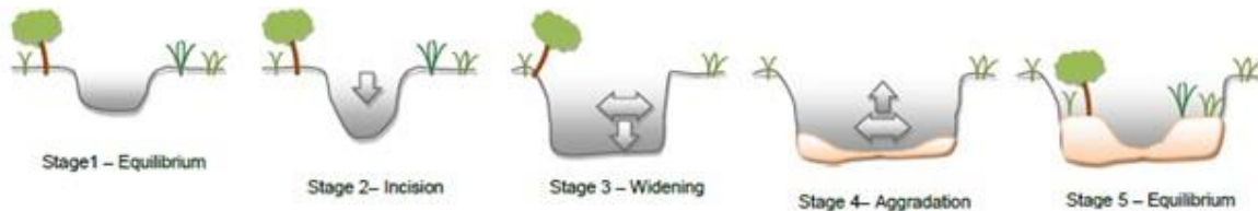
Figure 10: Channel evolution model (adapted from Schumm et al., 1984)
