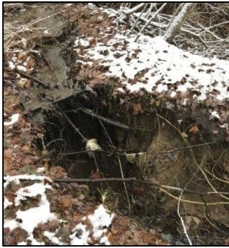
Figure 39: ~4-ft headcut in tributary
